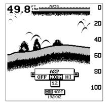
levels, try using the "High" ASP setting. However, if you are having trouble with noise, we suggest that you take steps to find the interference source and fix it, rather than continually using the unit with the high ASP setting. However, there are times when you may want to turn the ASP feature off. This allows you to view all incoming echoes before they are processed by the ASP feature.
